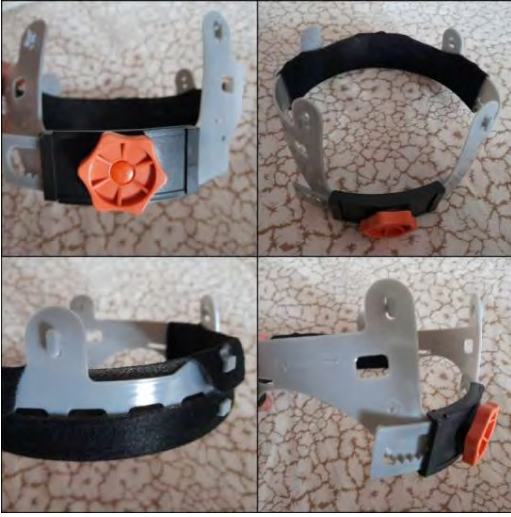
Fig. 5. Head mount used for the obstacle detection system.
