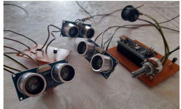
Fig. 4. The realized PCBs with the assembled components for the obstacle detection system.
